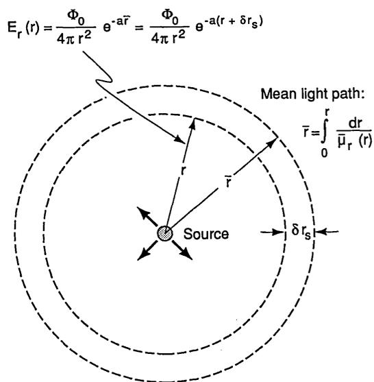
Fig. 2. Vector irradiance from an isotropic source embedded in a homogeneous scattering and absorbing medium.
