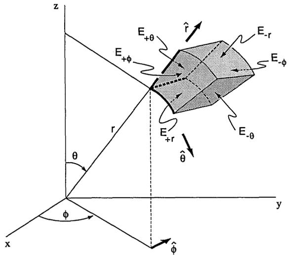
Fig. 1. Spherical components of vector irradiance. The three components of the vector irradiance are the differences of the irradiances incident upon the opposing faces.
