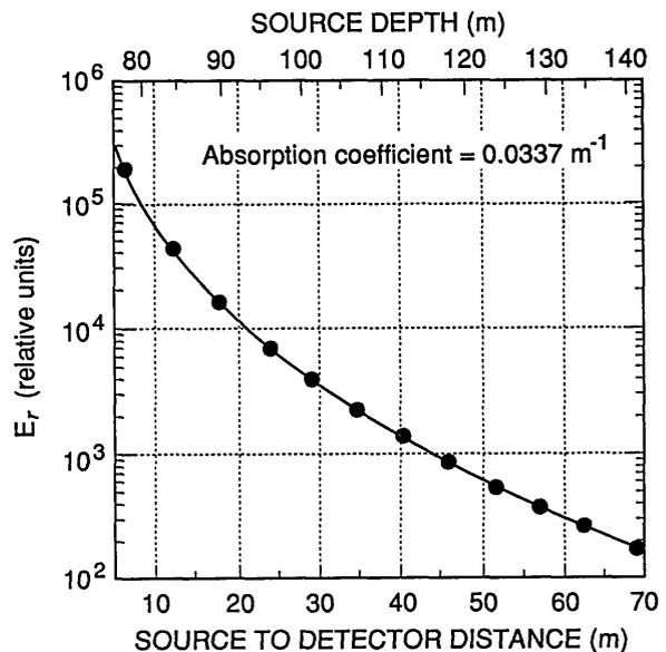
Fig. 3. Vector irradiance measurements from an isotropic source taken on 26 August 1990 off the coast of southern California.
