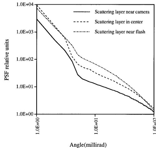
Fig. 2. Sample PSF's at  $\tau = 1.6$  for each scattering layer case.
