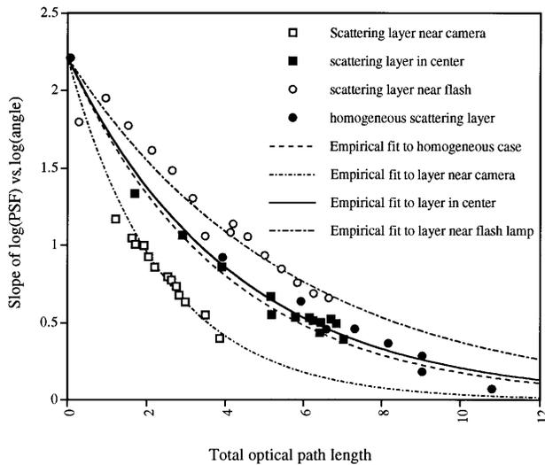
Fig. 3. Resulting slopes of  $\log(\text{PSF})$  versus  $\log(\text{angle})$  are shown as a function of optical path length, with the scattering layer in different positions. The most diffusing case, for the same path length, occurs with the scattering layer near the camera. Also shown is the empirical fit to the data in each case.
