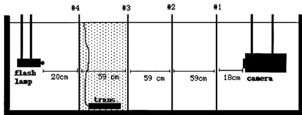
Fig. 1. Diagram of the experimental tank layout. The position of the flash-lamp source, receiving camera, and intervening Plexiglas dividers are shown; trans is the transmissometer measuring the beam attenuation in the scattering layer (in this case between separators 3 and 4, nearest the flash lamp).
