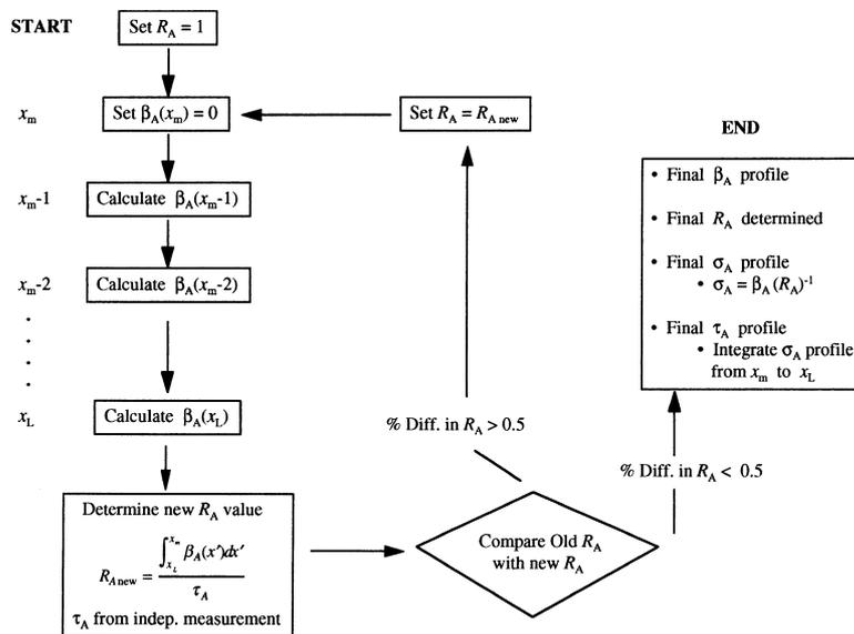
Fig. 12. Schematic representation of the lidar inversion algorithm.
