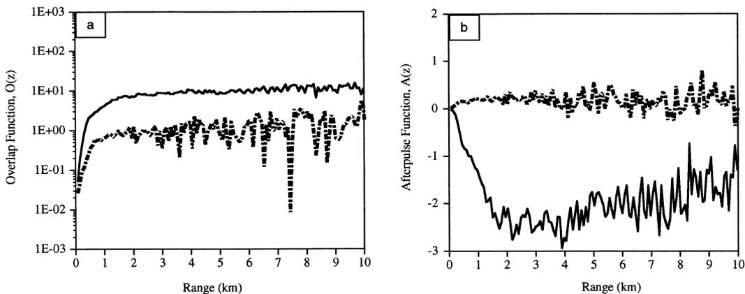
Fig. 2. (a) Overlap functions,  $O(z)$ , calculated on 29 June (solid line) and 15 July (dotted line) 1997. (b) Afterpulse functions,  $A(z)$ , calculated on 29 June (solid line) and 15 July (dotted line) 1997.
